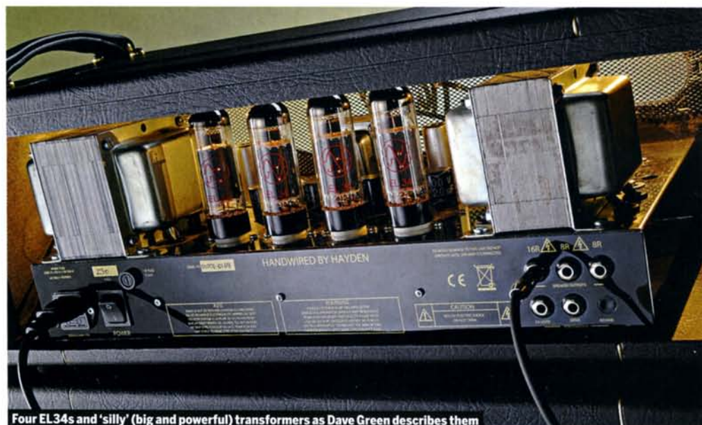
Four EL34s and 'silly' (big and powerful) transformers as Dave Green describes them
